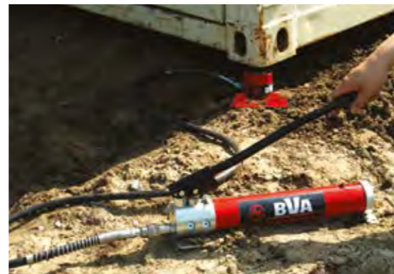
Low profile cylinders are great for confined spaces.
